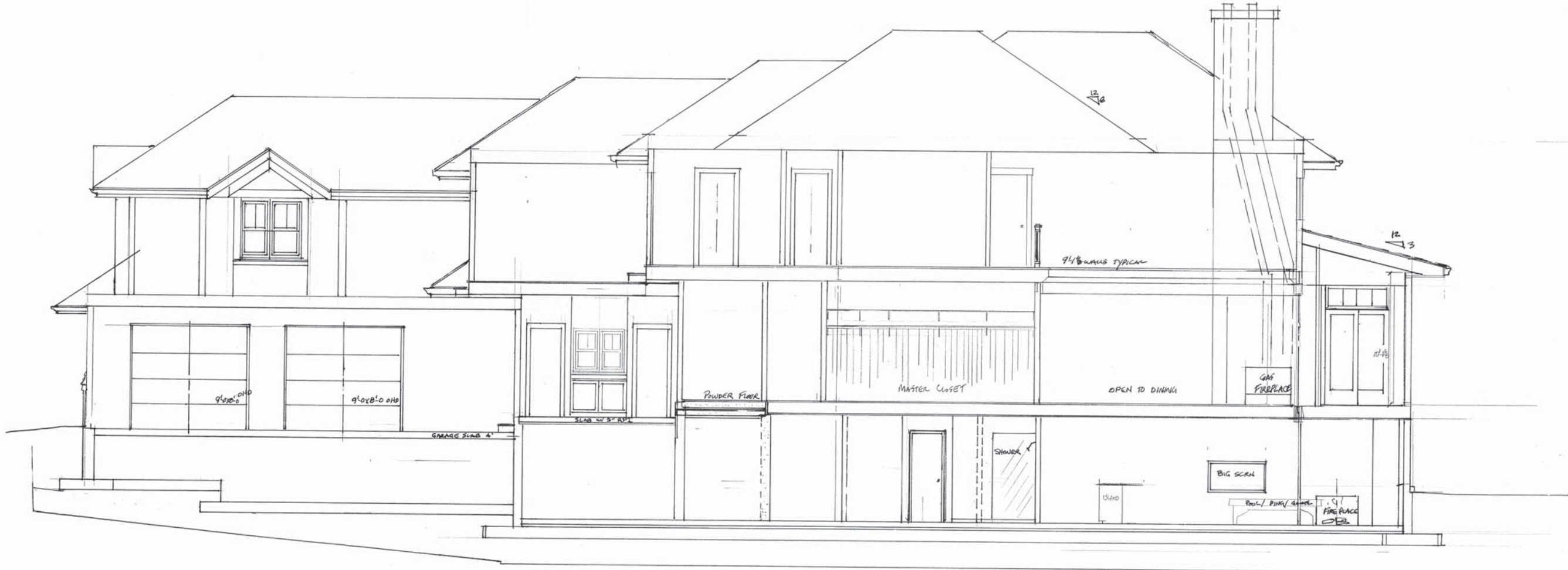
Section Thru "A-A" Scale 1/4" = 1'
