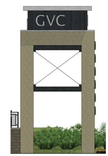
⑩ SIGNAGE TOWER WEST ELEVATION 3/16" = 1'-0"
