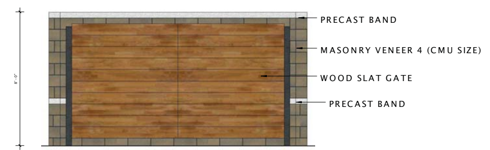
⑪ TRASH ENCLOSURE GATE ELEVATION 3/8" = 1'-0"
