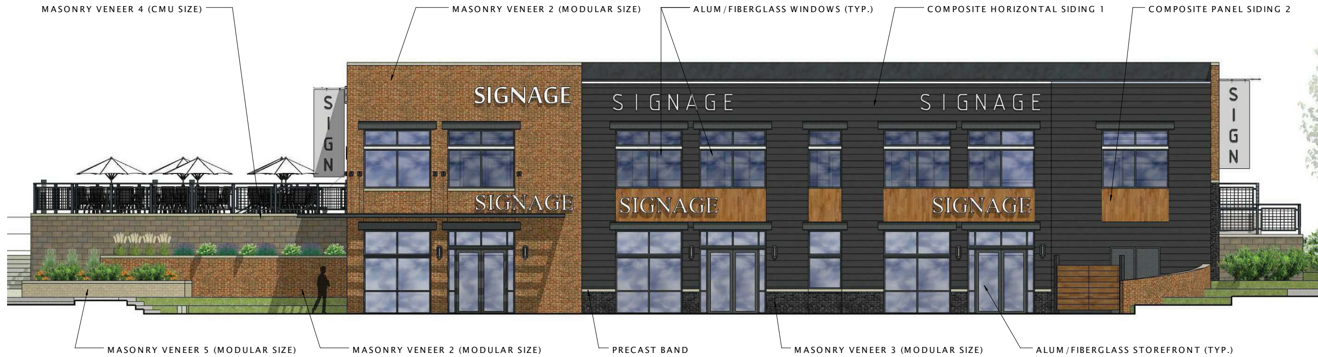
⑥ B3 SOUTH ELEVATION 3/16" = 1'-0"
