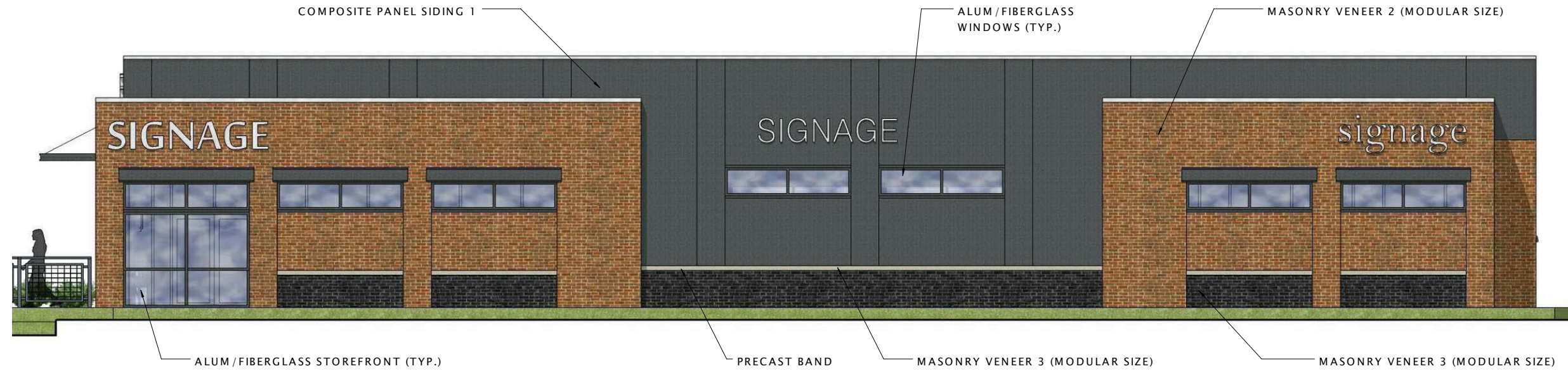
⑥ B4 SOUTH ELEVATION 1/4" = 1'-0"
