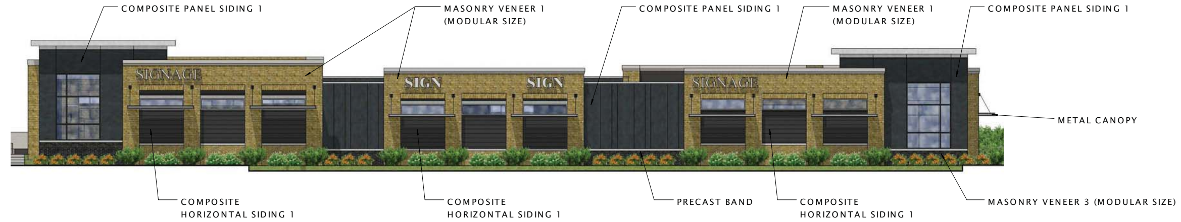
⑥ B5 SOUTH ELEVATION 1/8" = 1'-0"
