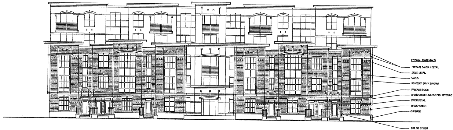
○ FRONT ELEVATION ALONG E. MIFFLIN STREET 1/8" = 1'-0"
