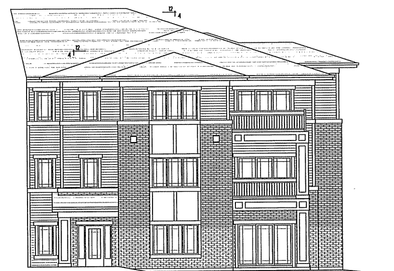
○ BUILDING A - INSIDE NORTH ELEVATION SCALE - 1/8" = 1'-0"
