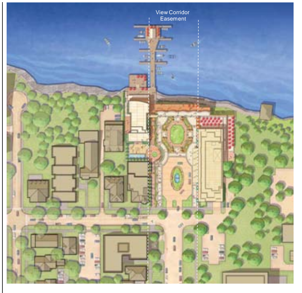
Figure 1.8 Site Plan Showing View Corridor Easement
