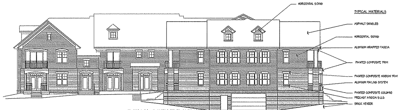
TYPICAL SOUTH ELEVATION WP - PDP
