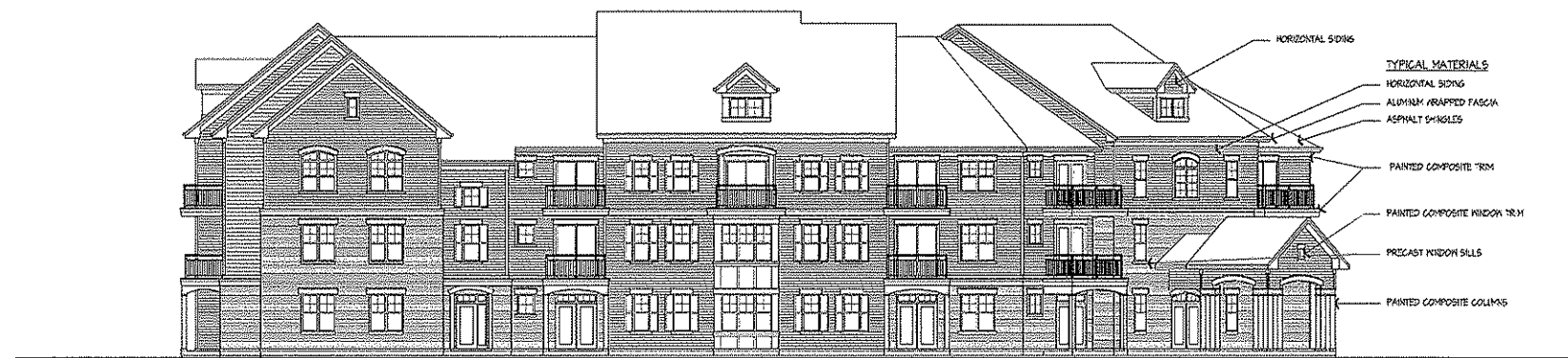
TYPICAL SOUTH ELEVATION 1/8" = 1'-0"
