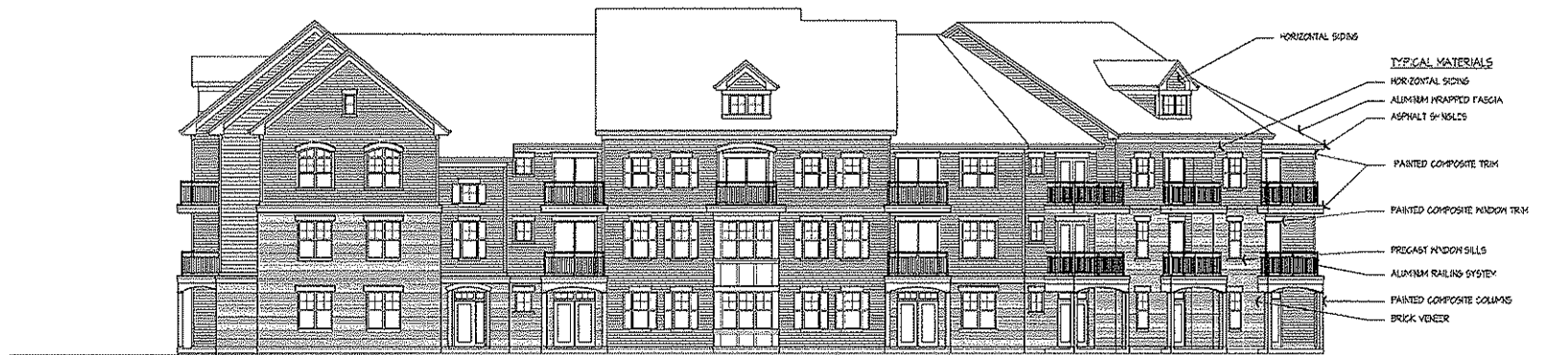
TYPICAL SOUTH ELEVATION 1/8" = 1'-0"
