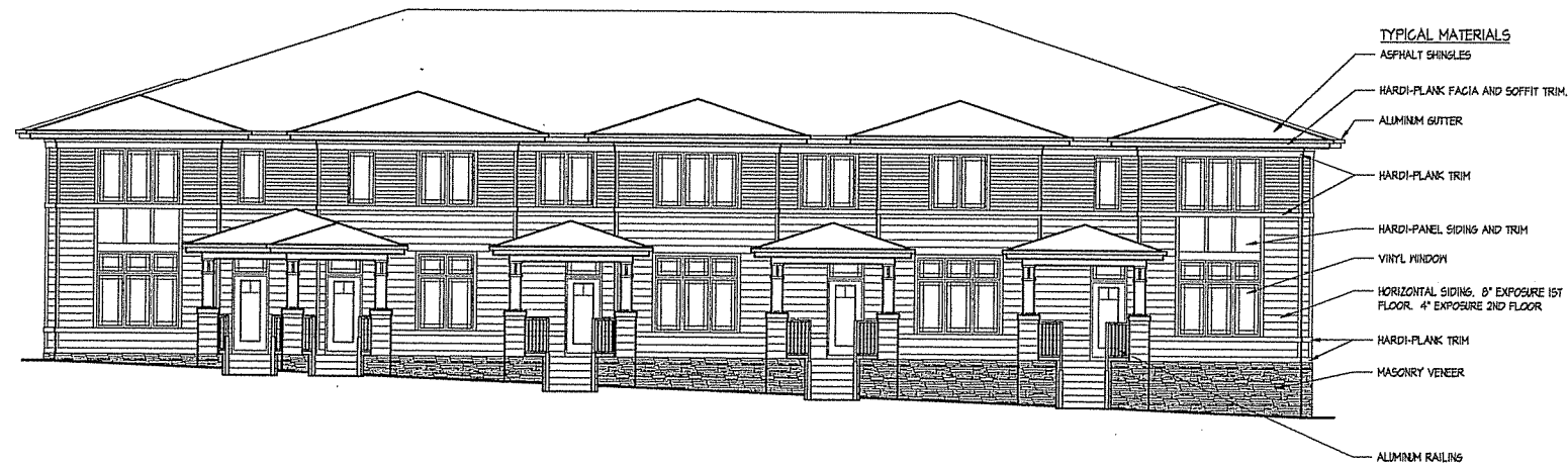
1 A-2.1 1/8" = 1'-0" TYPICAL FRONT ELEVATION
