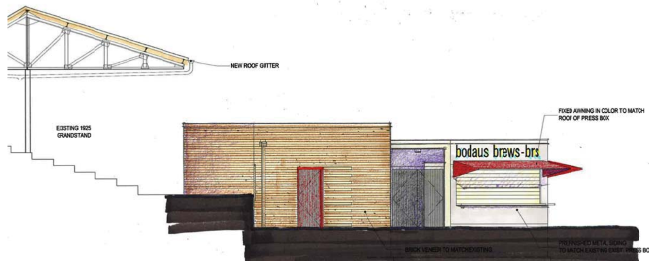
2 SOUTH ELEVATION - CONCESSIONS ADDITION Scale: 1/4"=1'-0"
