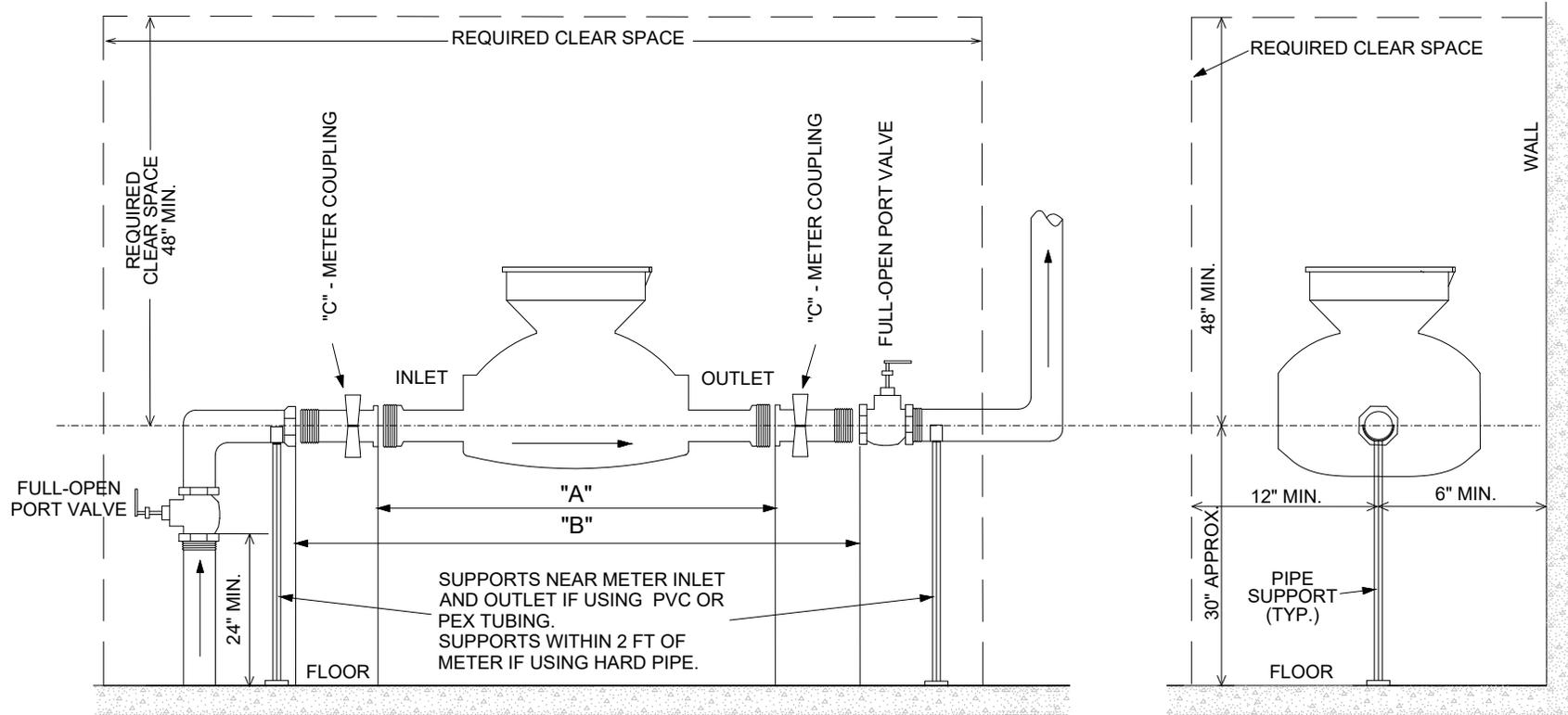
"A" - METER LAY LENGTH (BY METER SIZE):
