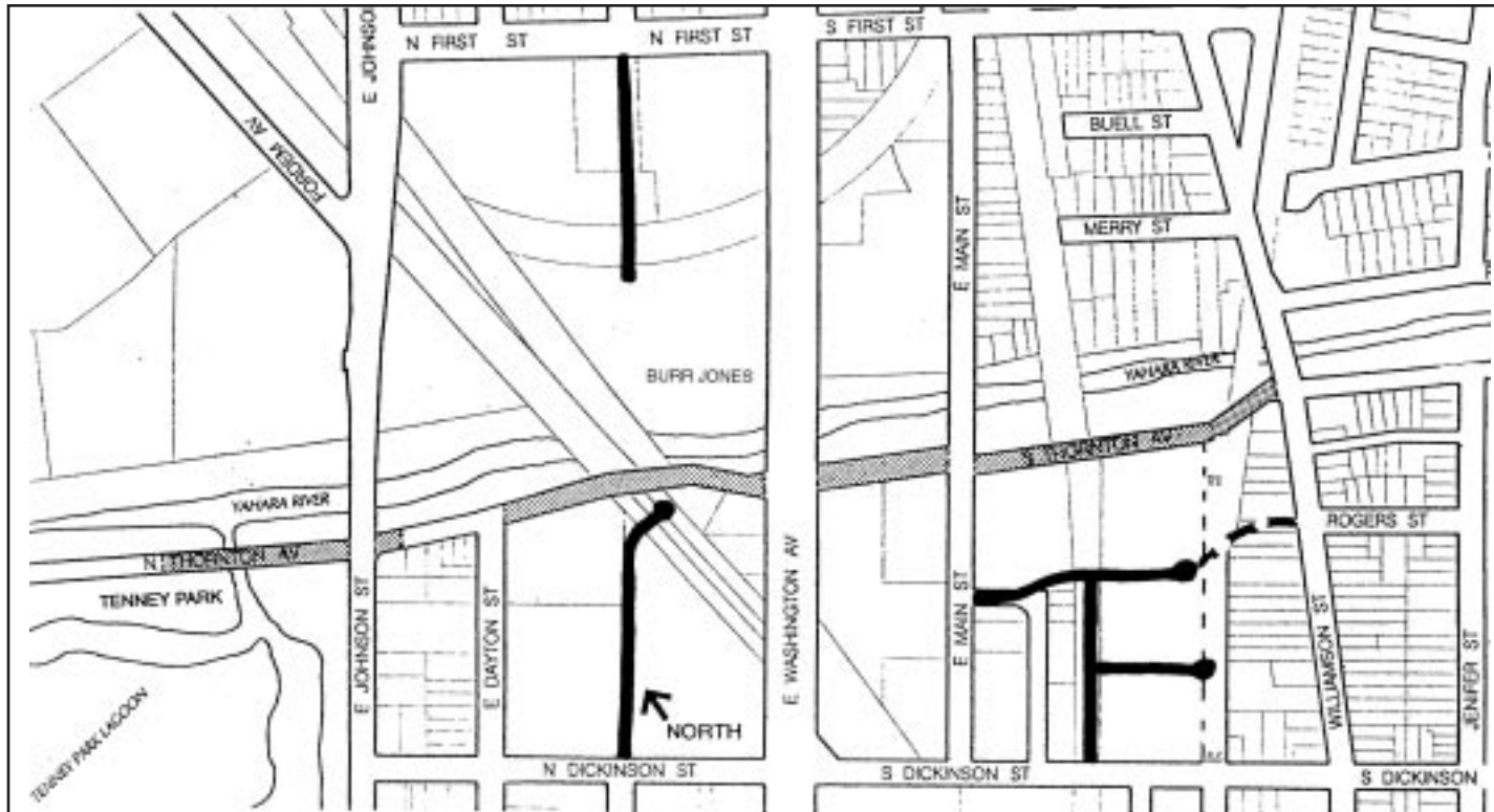
The gray areas locate parts of Thornton Avenue to be removed to create more park land, and the dark lines are potential streets to be added to aid neighborhood bike and vehicular circulation.
