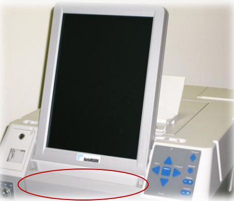
Pull Ballot Feed Tray up and out.
