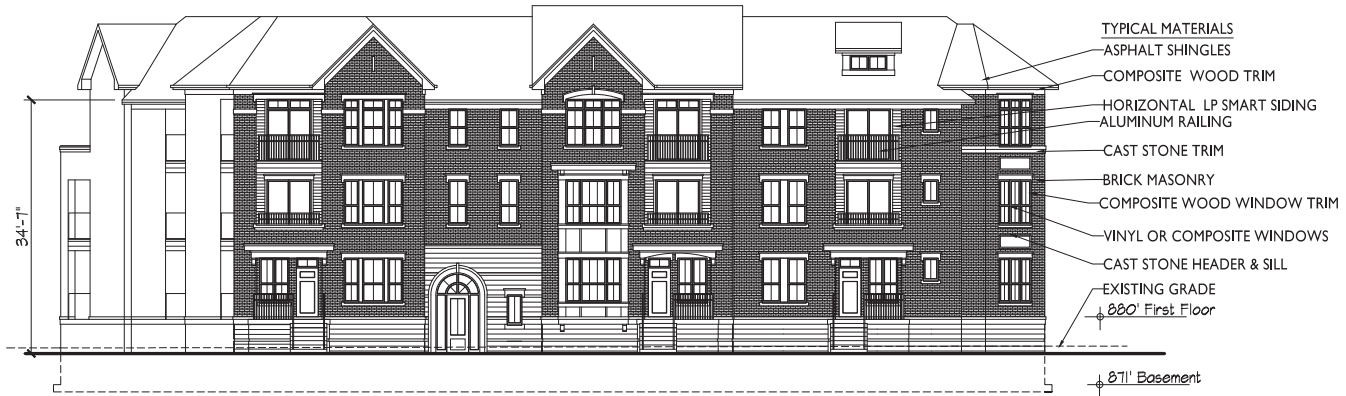
1 NORTH ELEVATION (ALONG UNIVERSITY AVE) A-2.1 108'-11-1/2"
