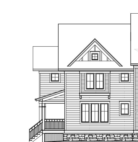
PARTIAL FRONT ELEVATION 1/8" = 1'-0" 7 UNIT TYPE "B"
